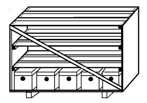
This crate can be made to move nuc boxes in multiple of five. It is a size that is easily made and handled. This crate can be loaded with a fork lift into a pickup truck or other well ventilated truck.
