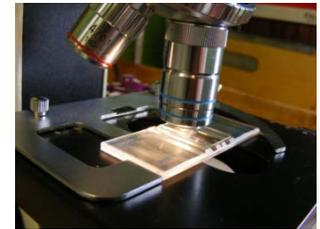
**7.** Starting on low (or medium) magnification place the slide under the microscope lens and focus on the grid of one chamber. Move to high power (400X) and then use the fine focus adjustment knob to avoid breaking the cover slip or slide.
