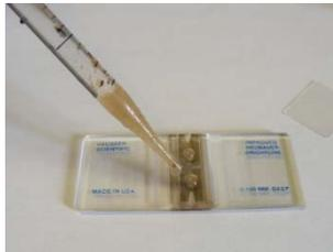
**5. Preparing the Slide:** Remove a sub-sample of the solution from the mortar (or vial) using the eyedropper. Avoid touching the walls or bottom of mortar/vial. Place a drop on each chamber of the hemacytometer.
