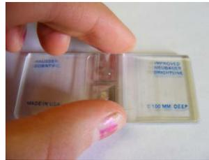
**6.** Place the cover slip on the hemacytometer. The solution will distribute evenly in the chambers. Allow the sample to settle for 1 to 2 minutes.
