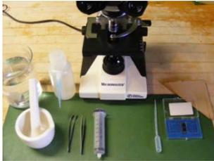
**Equipment:** forceps, mortar and pestle, clean water, 25mL syringe, eyedropper, hemacytometer and cover slip, 400X microscope, wash bottle, paper towel or soft cloth.
